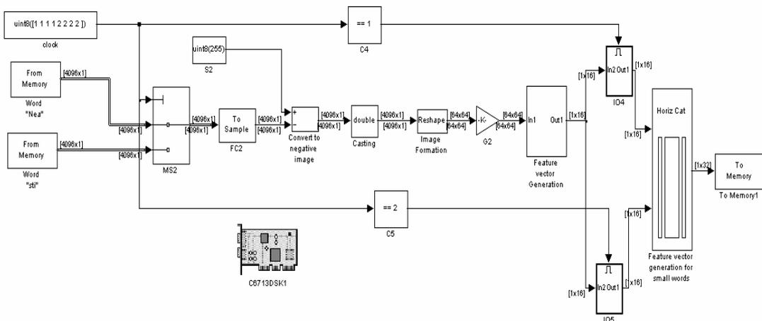
**Figure 4.** The image processing stage as imprinted in SIMULINK.
