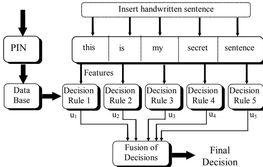
**Figure 2.** The proposed system architecture.
