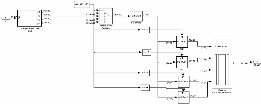
Figure 5. The segmentation procedure as it is imprinted in SIMULINK
