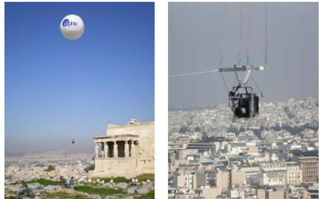
Figure 1. The balloon system (left) and the gyroscopic device mounted with the camera (right).
