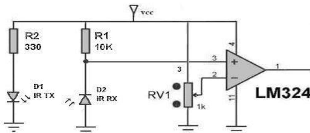
Fig.4 IR Sensor and Comparator circuit
