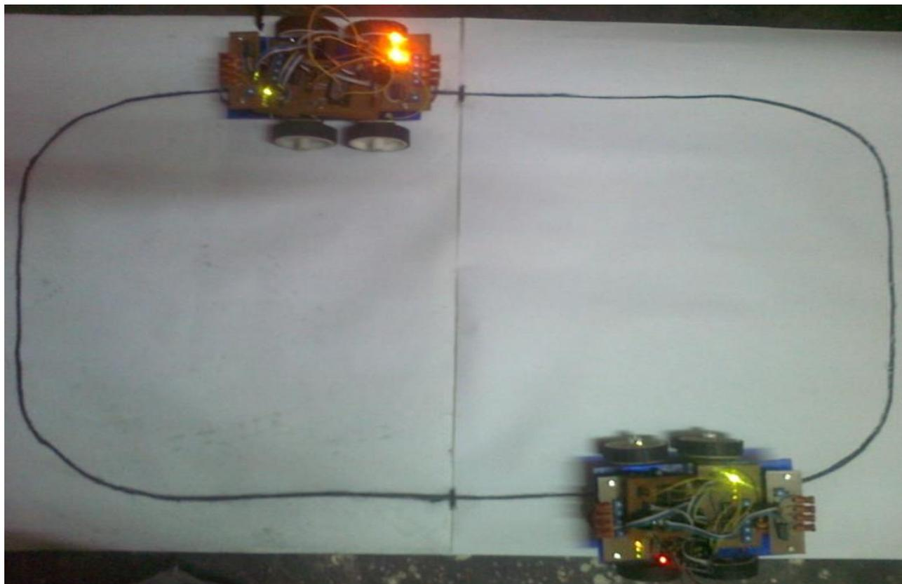
Fig.6 Relay Race Line Follower Robots
