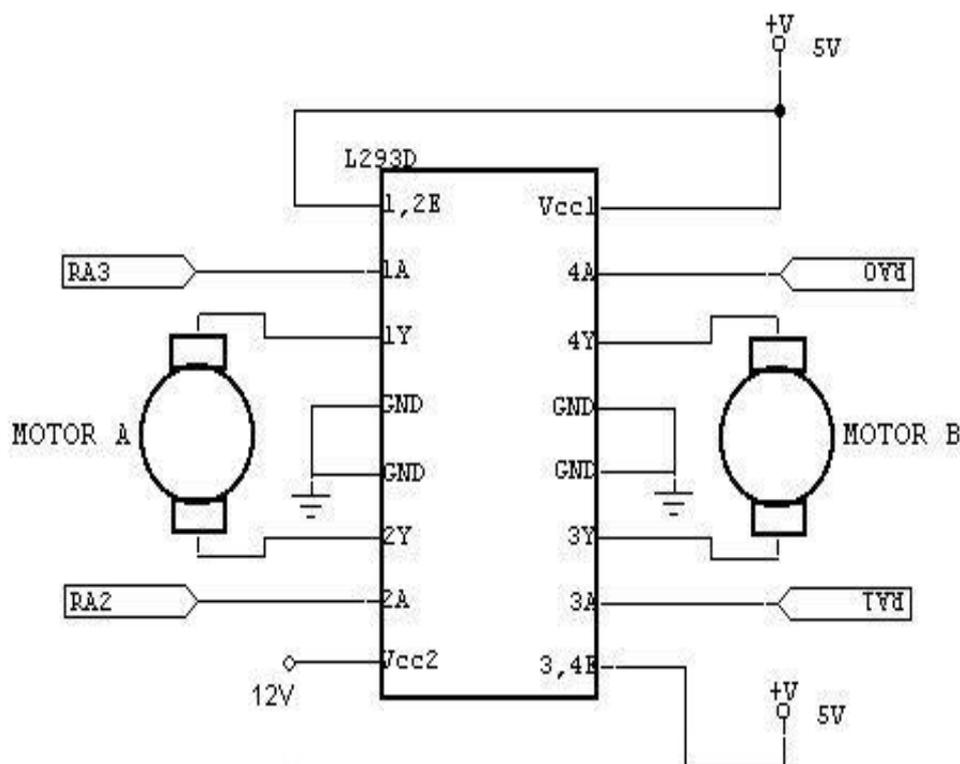
Fig.5 Driver circuit
